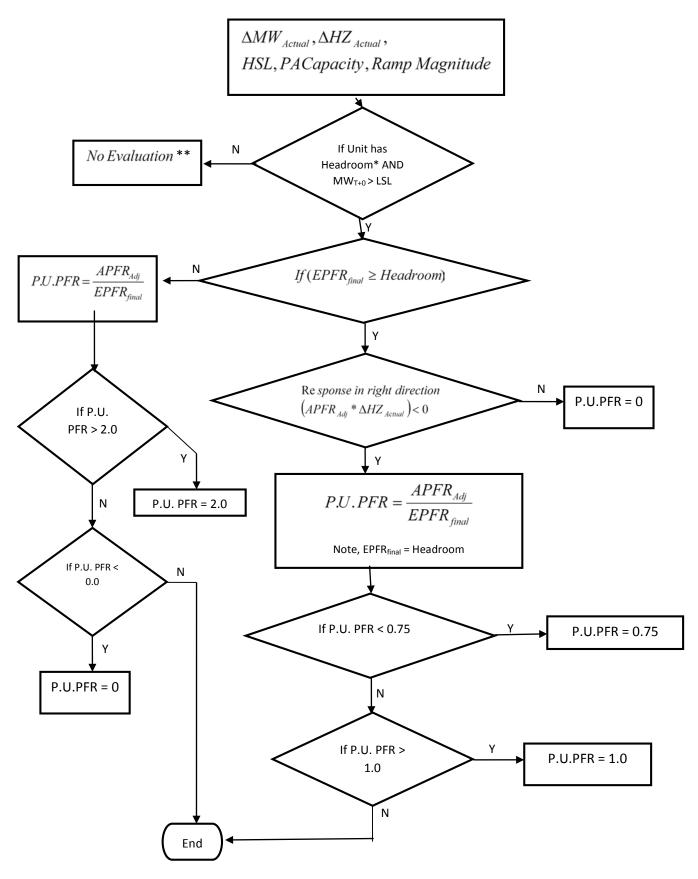
\*Check for adequate up headroom, low frequency events. Headroom must be greater than either 5MW or 2% of (HSL less PA Capacity), whichever is larger. If a unit does not have adequate up headroom, the unit is considered operating at full capacity and will not be evaluated for low frequency events.
